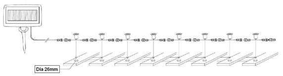
3. Insert each light through the hole by feeding the two wires through then pushing the light fixture firmly into place until it fits tightly against the deck surface (see illustration below). Repeat for all lights.
