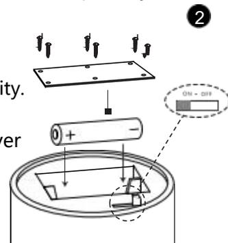
NOTE: Clean the battery contacts and those of the device prior to battery installation.
